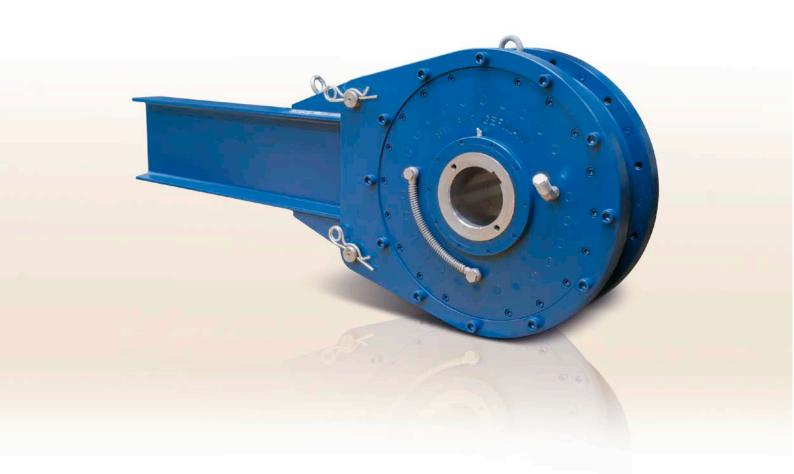
ackstops type RDBR-E are directly mounted on the drive shaft, e.g. of heavy duty conveyer belts, mixing drum drives and chain conveyors, when torque limiting / load sharing or the release function is required.
