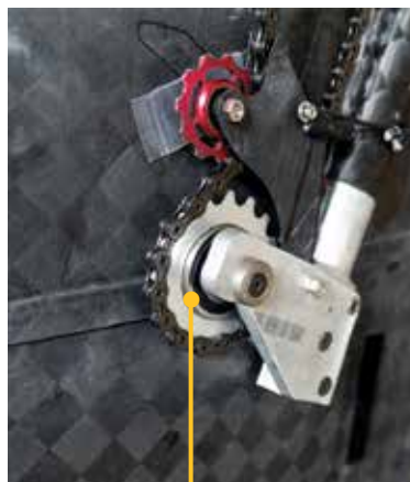
The Stieber CSK clutch was press fit onto the front wheel hub body, and pressed inside of the sprocket. It is responsible for driving the wheels up to 145 km/h (90 mph).
