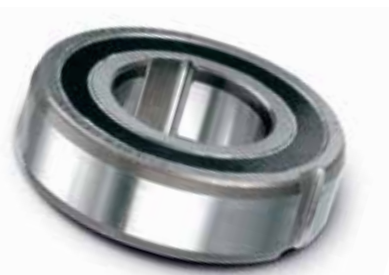
The Stieber Model CSK25 PP overrunning clutch features ultra-hard Formchrome® sprags which provide extra-long life, maximum wear resistance and lower maintenance costs. Formchrome sprags – exclusive to Stieber/Formsprag – are made by diffusing chromium into the surface of hardened high carbon alloy steel to form a chromium-carbide alloy.
